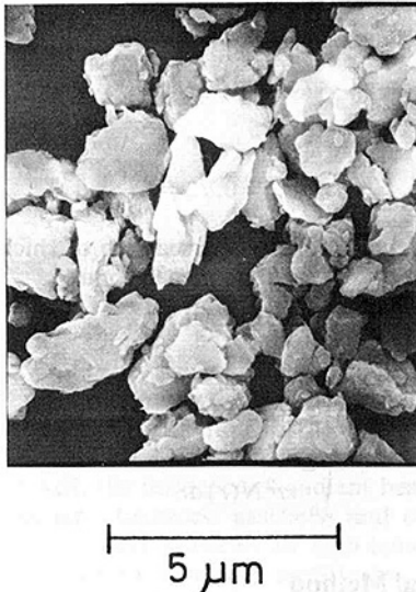
Fig. 1 Photomicrograph of coal (scale = 5 \mu\text{m} )
